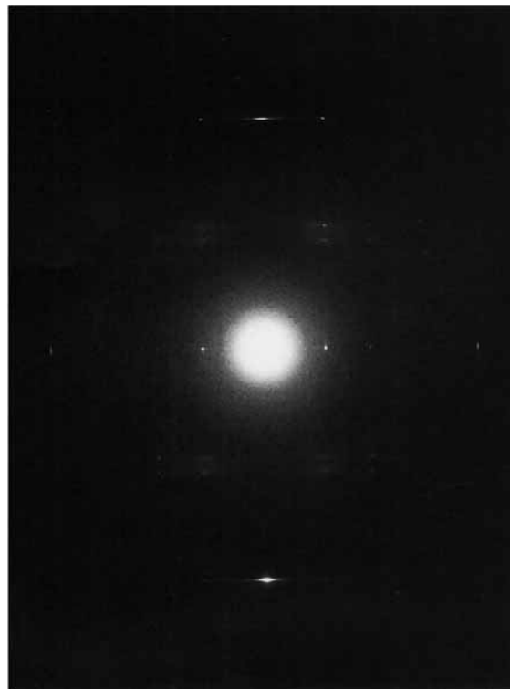
Figure 2 Electron diffraction pattern of a friction-deposited PTFE transfer layer. The friction direction is parallel to the meridional in the pattern.
